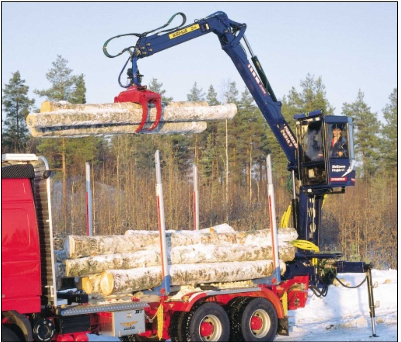
Foresteri 2010/2010T is a modern timber crane in the popular ten tonne-meter lift capacity class. With Foresteri 2010T you can handle full grapple loads at a radius of almost 10 meters.
