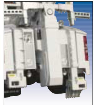
Full Hydraulic Independently Operated Rear Stabilizers Include Recovery Anchors
