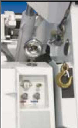
Boom Mounted Chain Storage Pockets & Recessed Auxiliary Hook-ups
